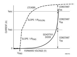
Figure 3. LTC4089/LTC4089-5 Versus Schottky Diode Forward Voltage Drop
