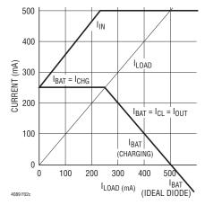
(c) High Power Mode with I<sub>CL</sub> = 500mA and I<sub>CHG</sub> = 250mA R<sub>PROG</sub> = 200k and R<sub>CLPROG</sub> = 2k
