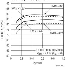
LTC4089-5 High Voltage Regulator Efficiency vs Output Load
