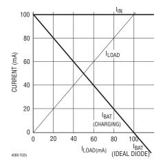
(b) Low Power Mode/Full Charge R<sub>PROG</sub> = 100k and R<sub>CLPROG</sub> = 2k
