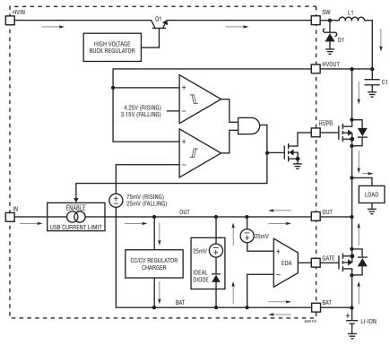
Figure 1. Simplified PowerPath Block Diagram
