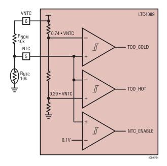
Figure 4. NTC Circuit
