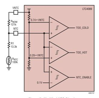
Figure 7. Modified NTC Circuit
