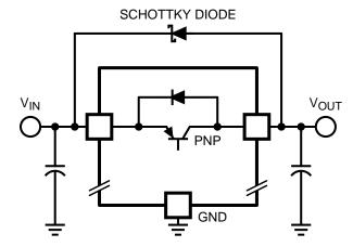
Figure 35. Adding External Schottky Diode Protection
