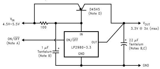
Figure 38. 5 V to 3.3 V at 3-A Converter
