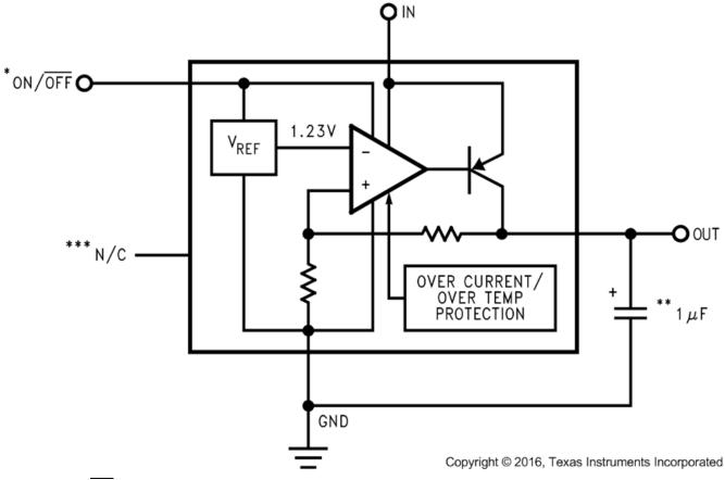
\*ON/OFF input must be actively terminated. Tie to IN if this function is not to be used.
