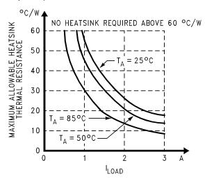
Figure 39. Heatsink Thermal Resistance Requirements for Figure 38
