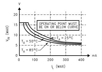
Figure 37. Safe Operation Boundary Curves for Figure 36
