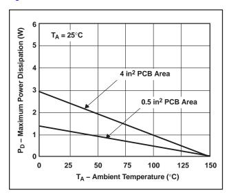
Figure 31. SOT223 Maximum Power Dissipation vs Ambient Temperature
