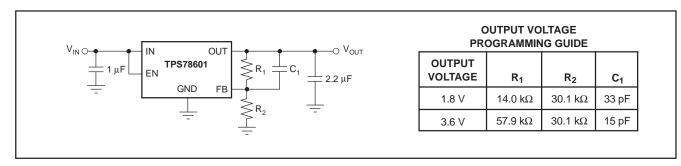
Figure 25. TPS78601 Adjustable LDO Regulator Programming
