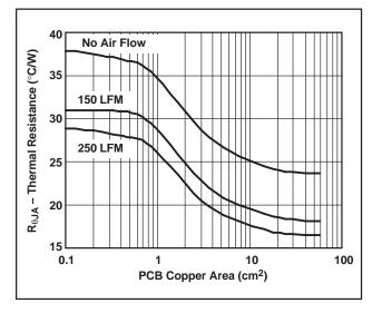
Figure 27. DDPAK Thermal Resistance vs PCB Copper Area
