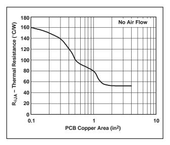
Figure 30. SOT223 Thermal Resistance vs PCB Copper Area
