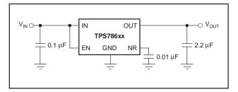
Figure 24. Typical Application Circuit
