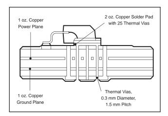
Figure 28. DDPAK Thermal Resistance Computer Model
